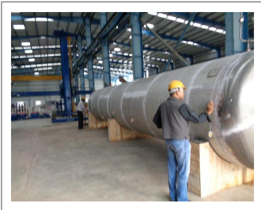
COLD STRETCH OPERATION UNDER PROGRESS FOR THE INNER VESSEL
