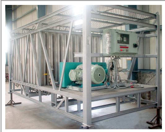
COMBINED PUMP & VAPORIZER SKID FOR HIGH PRESSURE PURGING & TESTING
