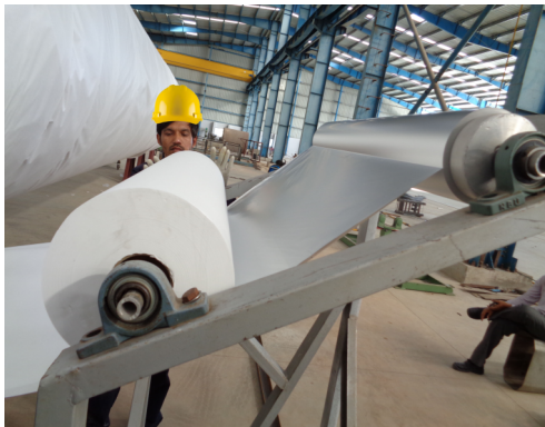
MULTILAYER INSULATION LNG TANKER WINDING IN PROCESS
