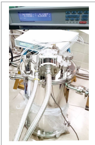
4.2 K CLOSED CYCLE REFRIGERATOR - ITER
