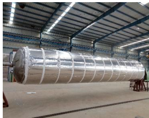
INNER VESSEL MULTILAYER WINDING WITH ALUMINIUM FOIL & IMPORTED GLASS PAPER
