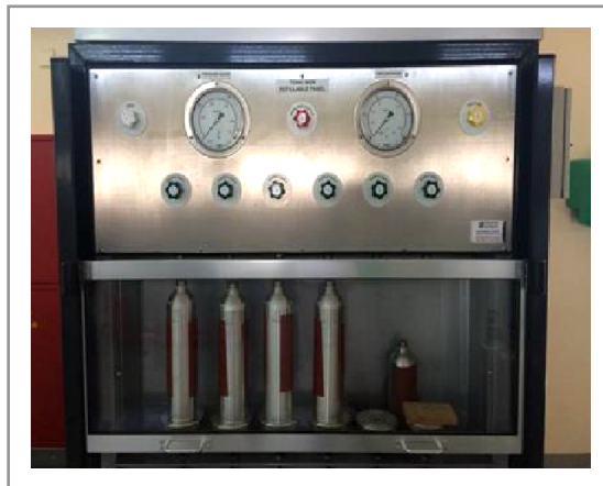
CANISTER FILLING STATION
