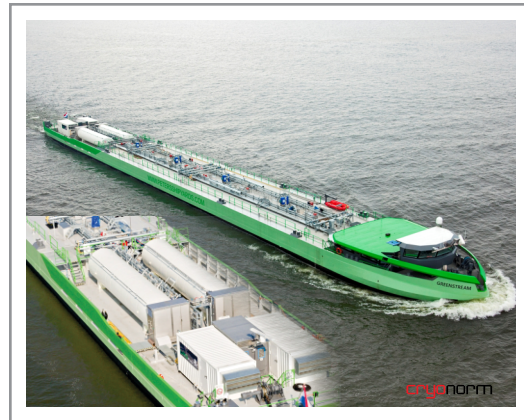
LNG STORAGE / RE-GAS FOR TWO INLAND PETROL TANKERS
