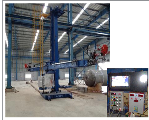
FULLY AUTOMATED CAMERA MONITORED SUBMERGED ARC WELDING SYSTEM
