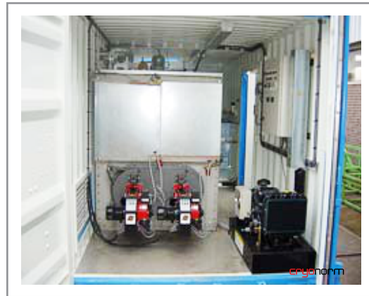
DIESEL FIRED VAPORIZER
