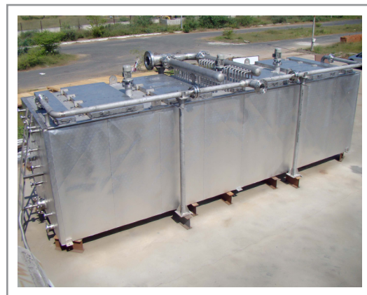
STEAM HEATED WATER BATH VAPORIZER
