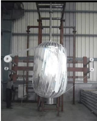
AUTO WINDING MLI ON MICRO BULK CRYOGENIC CONTAINERS
