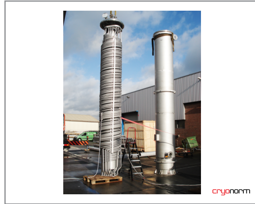
HOT WATER HEATED VAPORIZER
